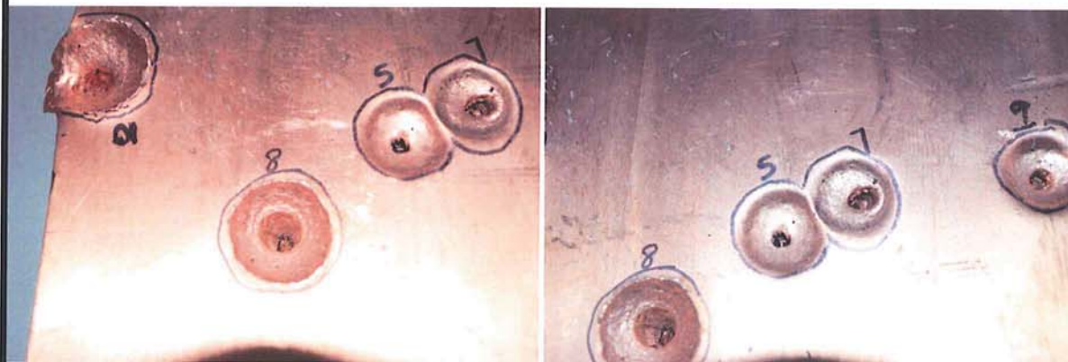
Figure 2 - Close-up views of copper target specimen with projectile damage zones
