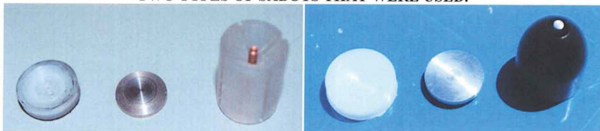
Figure 1 - The bullet-shaped sabot on the right was modified in a variety of different ways to create a vented sabot, a split sabot, and a solid sabot with a variety of different mouth openings and tightnesses of fit against the rod.
