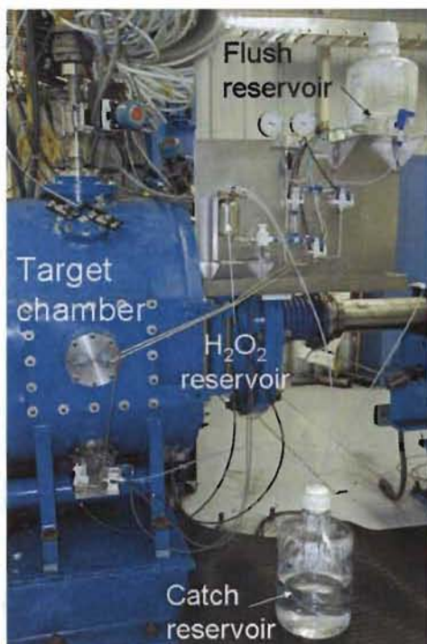
Figure 5. RLLS is shown as implemented on the LANL two-stage gas gun. The \text{H}_2\text{O}_2 reservoir and several valves are located on a plate situated so that the components are above the target cell inside the target chamber to facilitate a gravity feed to the cell. There is also a large container of water on the plate that allows flushing the system after an experiment.
