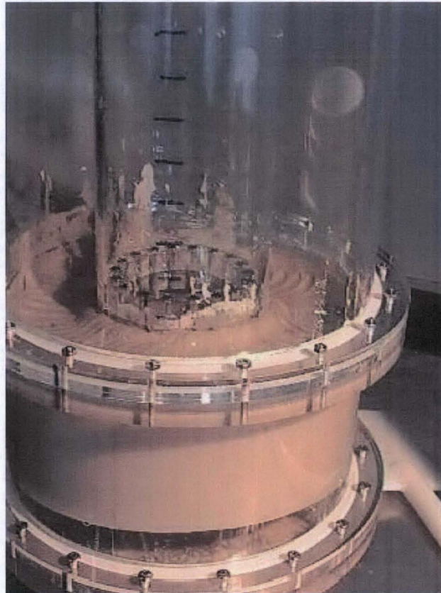
Figure 3-3 Stable rising annular sludge plug.
