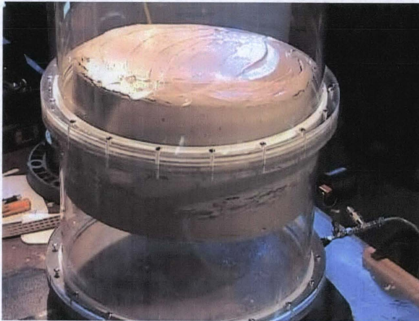
Figure 4-3 Strong sludge plug ( > 1600 Pa) rising through contraction established by sludge buster shelf located at flange. The extruded portion of the sludge plug above the shelf has separated from the container wall. Failure occurred after about two-thirds of the plug was extruded.
