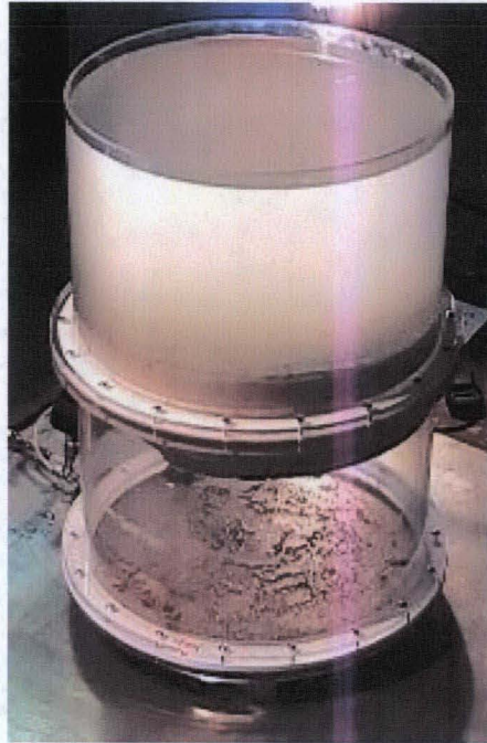
Figure 3-12 Stable three layer configuration in cylindrical container (vessel spanning bubble + sludge layer + water layer).
