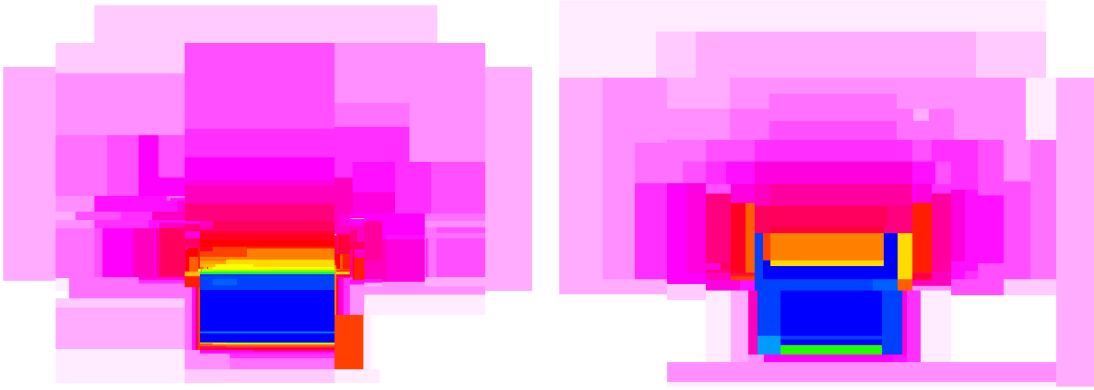
Figure 6. kd-tree representations of electron-range data generated with bin-based algorithms.
