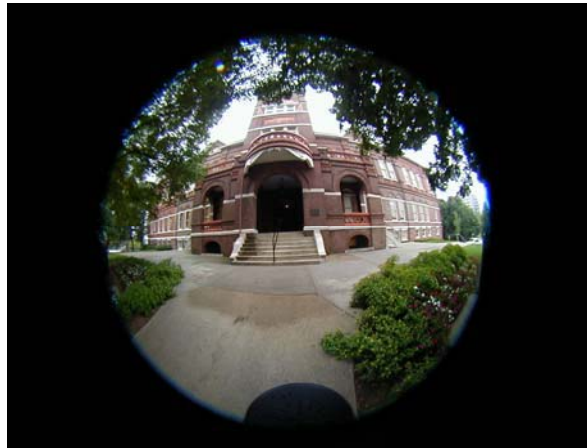
Figure 1: Sample of raw image taken with an IQInvision IQEye3 camera configured with an IPix fisheye lens. The image area is 360 degrees by 180 degrees in scope. The image is 1.3 megapixels in resolution. (Note: image used is from the IPix Software Development Kit sample package.)
