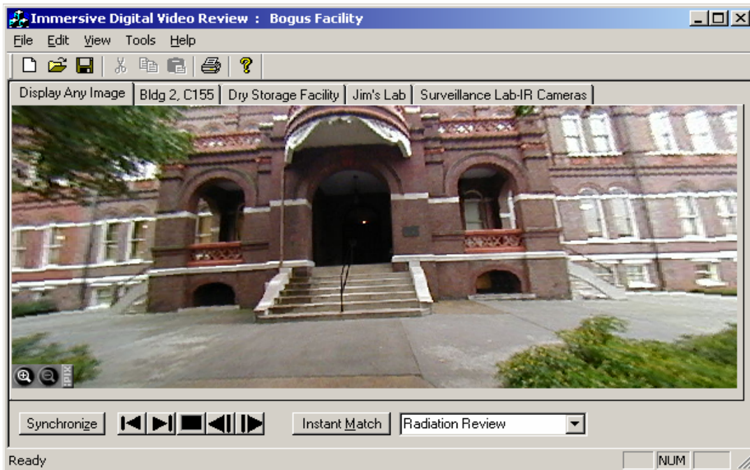
Figure 2. Fisheye image displayed in an immersive viewer developed by Los Alamos National Laboratory, using the IPix software development kit. The image is de-warped and the viewer software provides the ability to virtually pan, tilt, and zoom within the context of the image. The image is 1.3 megapixels in resolution.
