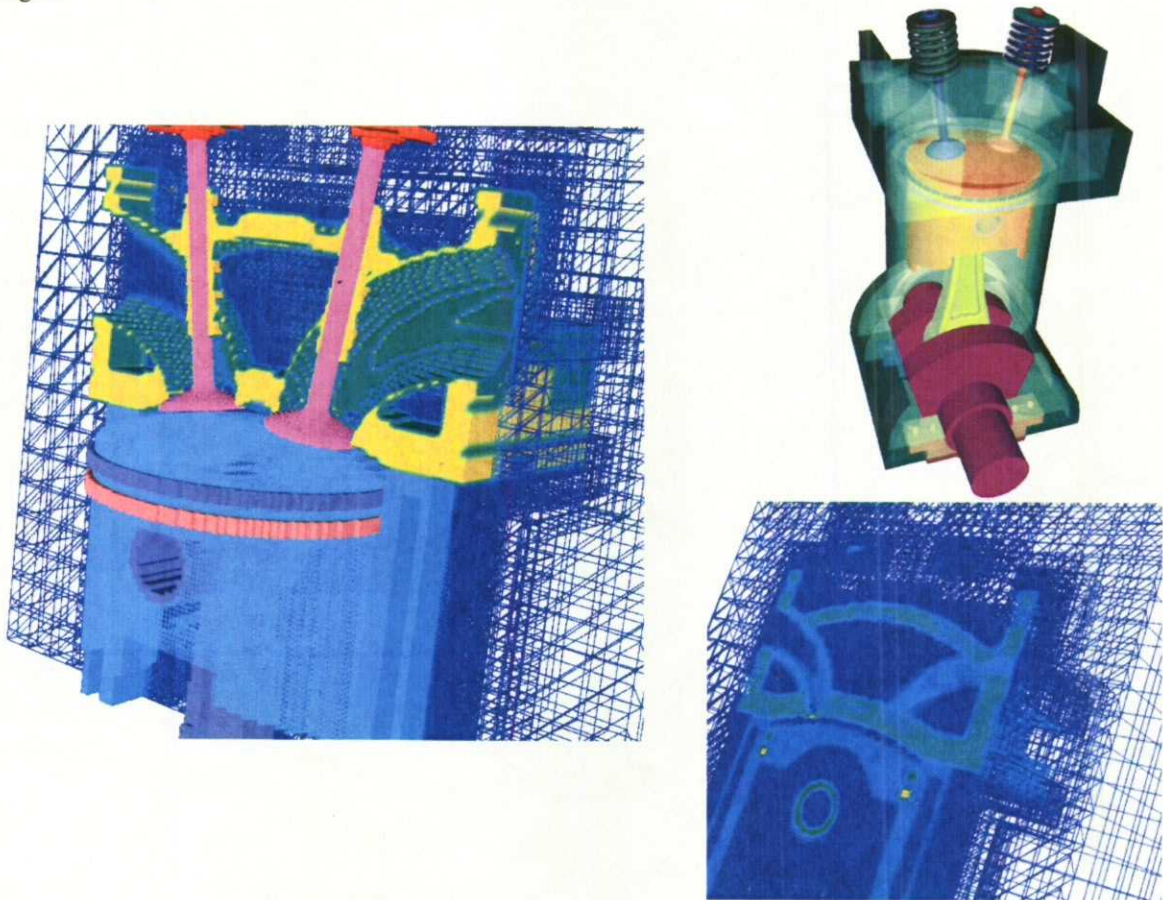
Fig. 1. An example of the use of CAD/CAM 3D solid geometry modeling to generate a continuous adaptive mesh refinement mesh for a portion of a piston engine.
