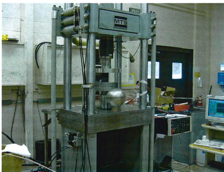
Figure 4: SwRI 200 kip load frame and float testing apparatus.
