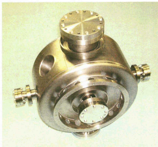
Figure 5: LANL/AAA \beta = 0.175 , 2-Gap, 350 MHz Cavity
