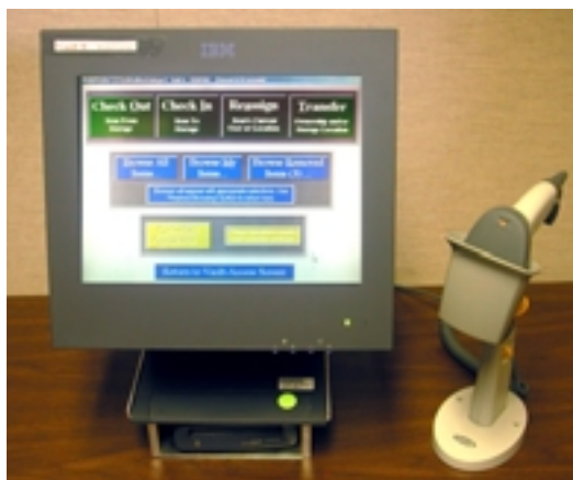
Figure 1. Touch screen CPU, a laser bar code scanner, and the MediaTracker software provides media tracking at the entrance of the vault/VTR.
