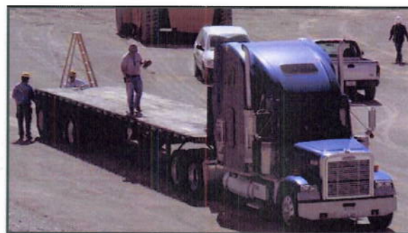
Once mixed low-level waste packages are unloaded, a radiological survey is conducted on all truck trailers prior to release from the NTS
