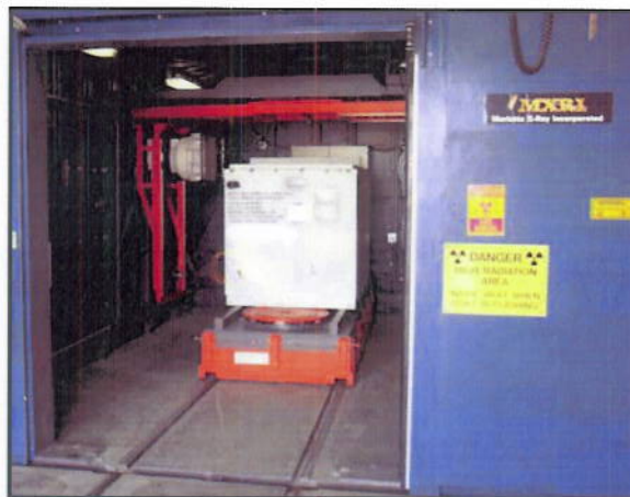
The existing RCRA Part B Permit requires a percentage of mixed low-level waste disposed at the NTS be visually examined using x-ray technology
