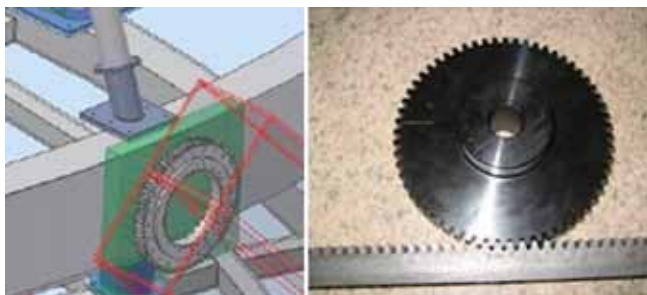
Figure 5. The left figure shows a model of the bearings and gear for an elevation drive system. The right figure is a design for a low-cost, fast-rotating telescope, azimuth drive motion system.
