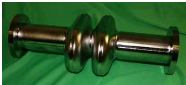
Figure 3. Model of a 2-cell niobium RF-deflecting cavity.
