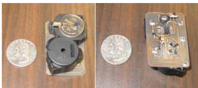
Figure 1. Both sides of the preliminary acoustic chirper tag and real-time monitor developed in FY09, which has not been fully miniaturized.
