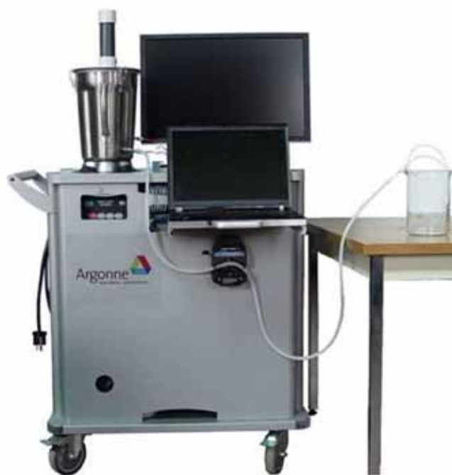
Figure 2. Argonne computer-automated, portable medical ice slurry production/delivery system.
