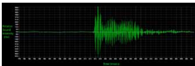
Figure 2. Chirp waveform generated by the device shown in Figure 1, as recorded by a microphone.
