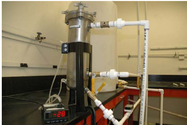
Fig. 59 Close up picture of the filter and pressure transducer
