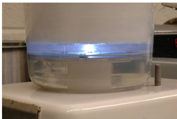
Fig 40 Spark discharge produced by pinhole discharge using a nano-second pulsed power supply
