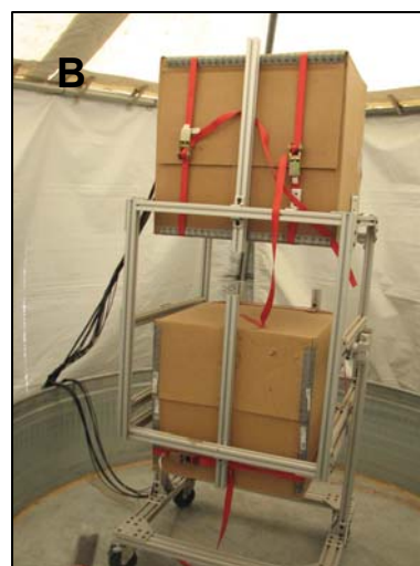
Figure 4. (A) Container and tent from which upward and downward looking measurements were respectively taken. (B) Neutron scatter camera taking downward measurements from inside of tent at a water depth of 0 cm.
