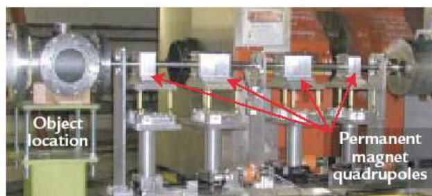
Figure 5. The microscope in the beamline. Large red objects in background are big quads A and B.
