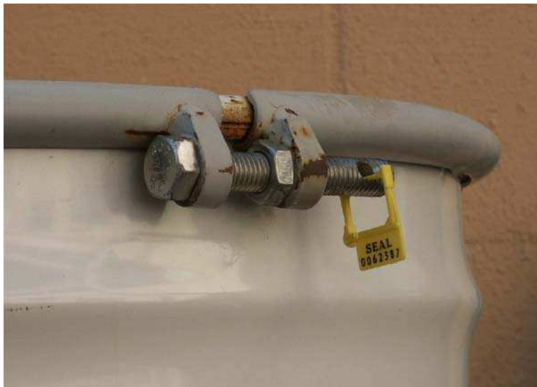
Figure 4 - An example of using a seal on a 55-gallon drum for low-security applications.
