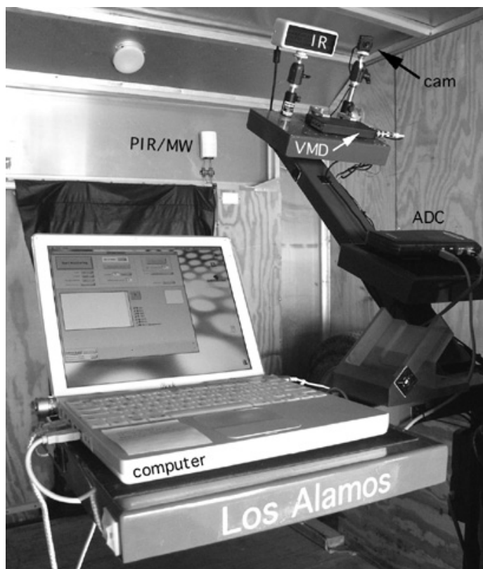
Fig. 3. A close-up of the Sender computer and some of the monitoring hardware.
