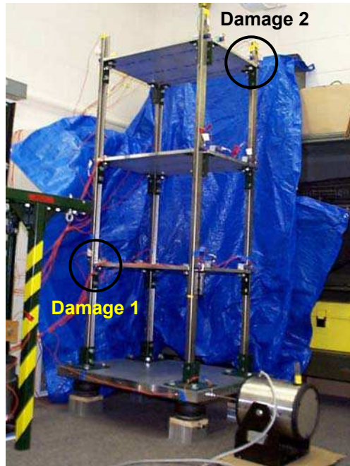
Figure 1: a three-story frame structure with dimension and damage locations
