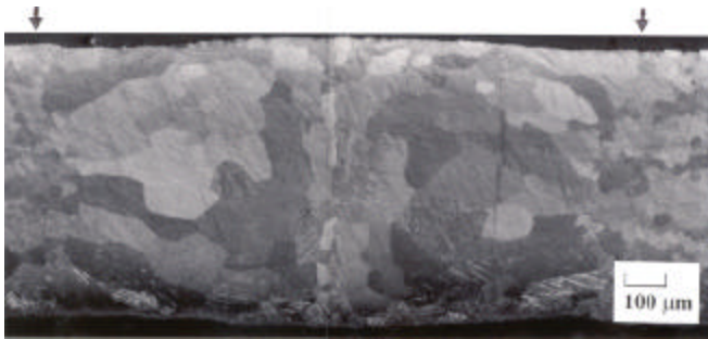
Figure 19. Near full penetration laser weld in rhenium displaying large grain growth and reduced occurrence of porosity.
