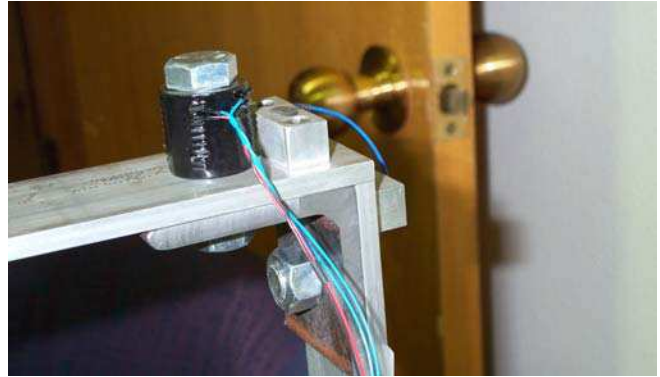
Figure 4: PZT washer stack used to vary preload in the bolted connection.
