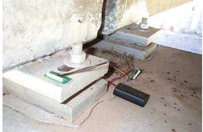
Figure 8: Accelerometers and processing board mounted on bearing plate under a bridge girder at a pier.
