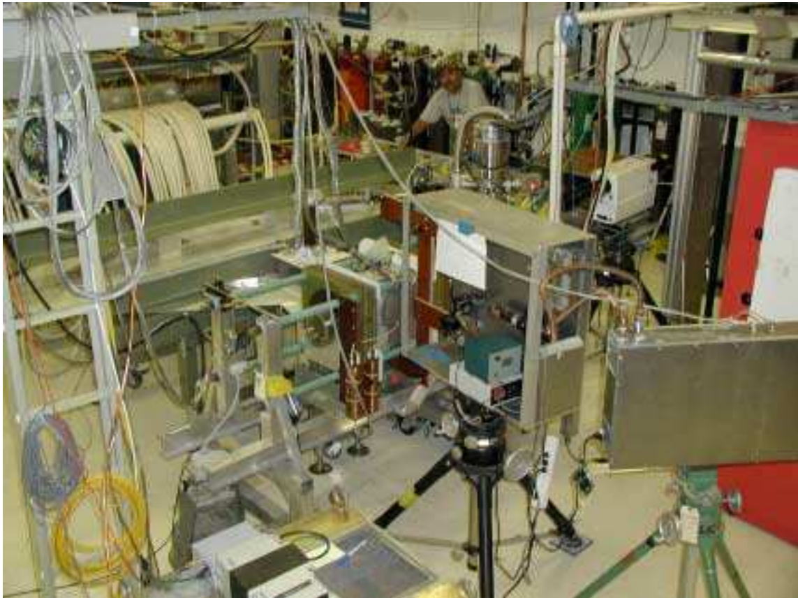
Figure 3: A recent picture of the new FRX-L laboratory, with the FRX-L FRC in the middle of the photo, partially hidden in the foreground by the 3.39 micron laser interferometer, and in the background by the fan-shaped parallel-plate header which feeds currents to the 1-turn theta-coils.
