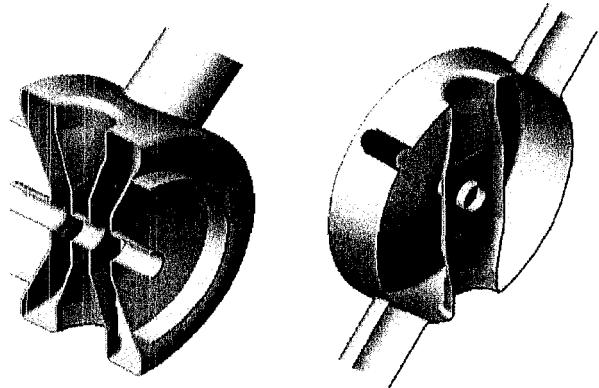
Figure 2: This is a cut-away view of the final cavity geometry with optimized spoke shape, all attached ports and the selected end-wall geometry.
