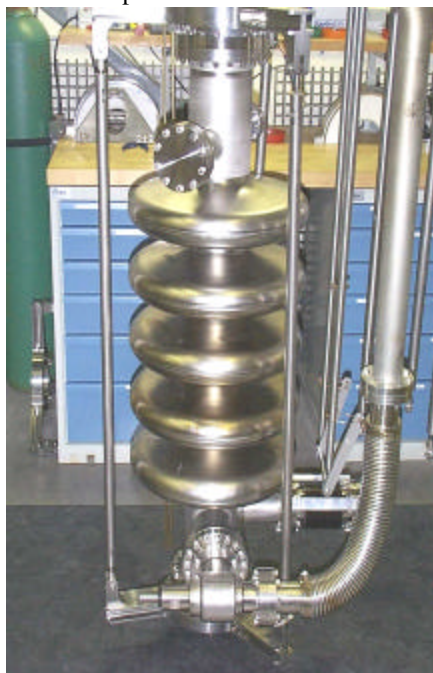
Figure 1: APT 5-cell cavity set on the cryostat insert. Details of the tests are described in [2-4].
