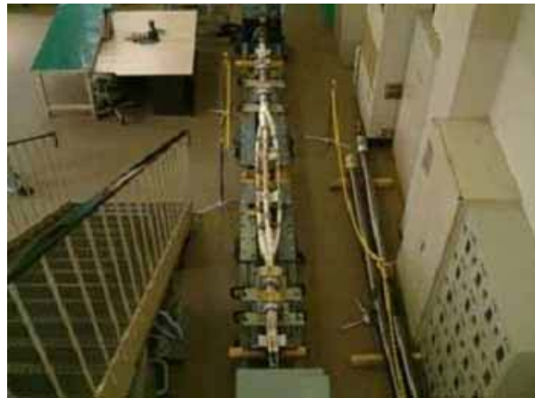
Figure 22 Tension Test of Three Phase Cable-to-Cable Joint
