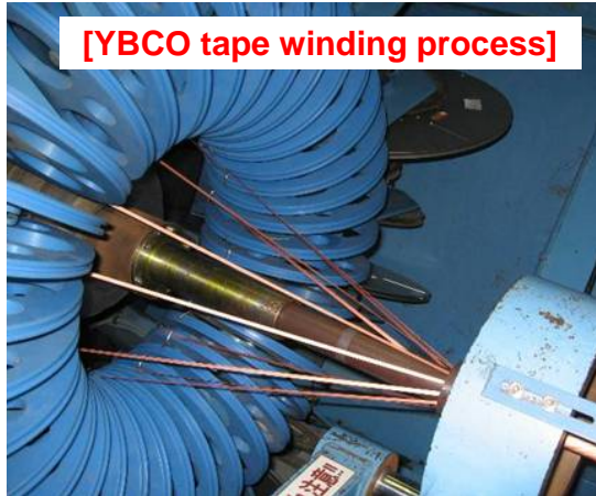
Figure 58 YBCO Cable Fabrication.
