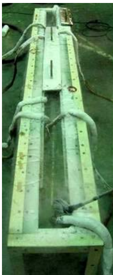
Figure 53 1 m YBCO 3 Core Sample Test Setup and Critical Current Results.
