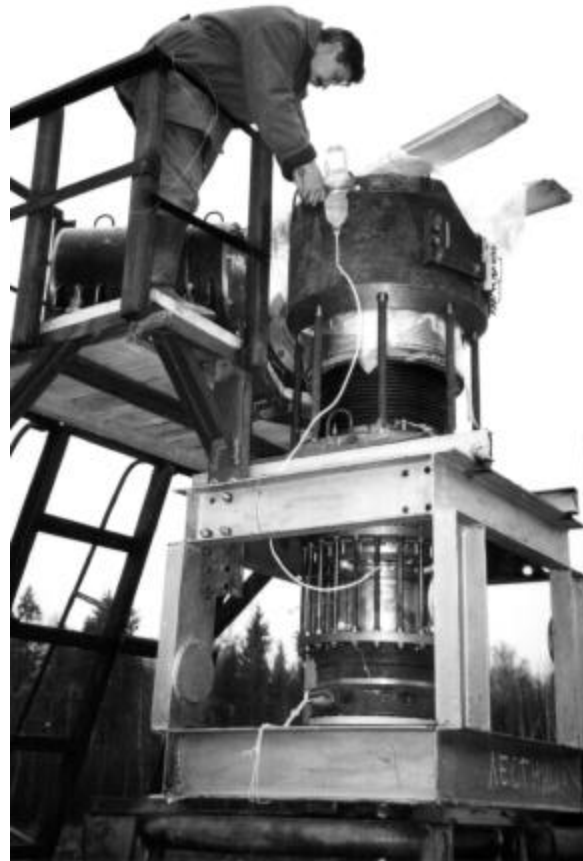
Figure 1. Photograph of the ALT-1 device on the firing point. The disk explosive electromagnetic generator (DEMG) is visible inside the heavy steel frame. Above the frame is the cylindrical transmission line, and above that is steel shielding surrounding the imploding liner experimental unit. Two radiographic x-ray sources are to the left of the shielding. Below the generator, not visible in this photograph, is the explosive driven helical electromagnetic generator (HEMG) that provides seed current for the disk generator.
