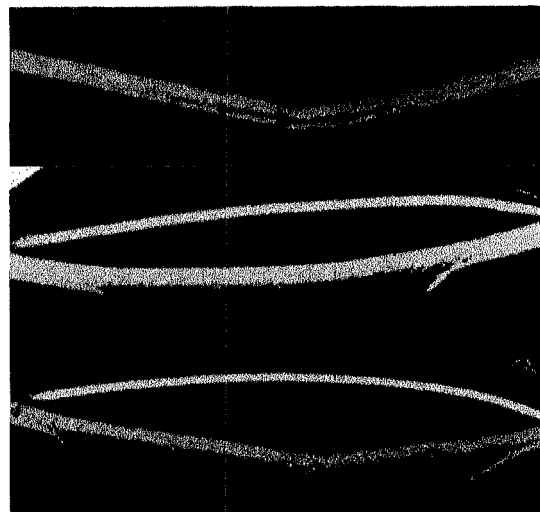
FIGURE 4 Post-shot metallography photographs of electro-refined (high-purity) uranium spall shots with peak free surface velocities, 371, 385, 413 m/s, from top to bottom.
