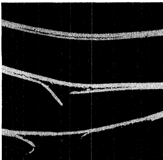
FIGURE 3 Post-shot metallography photographs of rolled uranium foil spall shots with peak free surface velocities, 322, 353, and 399 m/s, from top to bottom.
