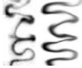
Figure 4. \text{SF}_6 volume fraction at 400 \mu\text{s} for the experimental image (left) and the first-order Cuervo result (right).
