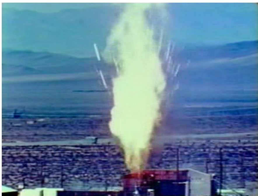
Figure 2-7 Kiwi - Upset Operation Source: LASL, 1962
