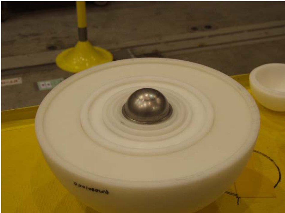
Figure 3: Photograph of the plutonium source in the nested HDPE hemishells
