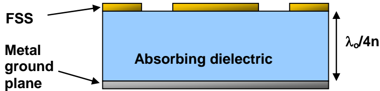
Figure 21. A representative unit cell for an infrared antenna. Absorbing dielectric thickness is roughly one-quarter of the freespace design wavelength divided by the index of the material. Dielectric can be a detector material such as HgCdTe.
