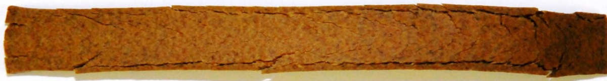
Figure 40. Photograph of an injection molded PHB/WF composite (control formulation, immersed for 4 days) (Anderson, 2007).
