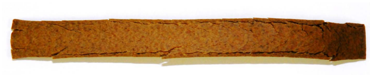
Figure 25. Specimen photograph of PHB/WF composite depicting cracking damage occurring during water absorption experiments. All specimens experiencing such damage were noted.
