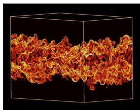
**Direct Numerical Simulation of Turbulent Nonpremixed Combustion. Instantaneous isocontours of the total scalar dissipation rate field.** (From "Direct Numerical Simulation of Temporally-Evolving Plane Jet Flames with Detailed CO/H<sub>2</sub> Kinetics," submitted to the 31st International Symposium on Combustion, 2006.) **Simulation performed at NERSC by Dr. J. Chen and coworkers.**
