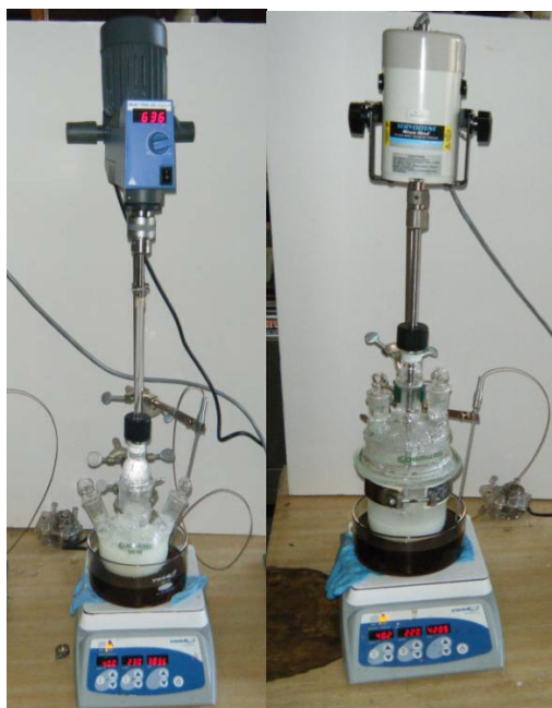
Figure 3 – Reactor testing systems (6 systems obtained for parallel studies); QCM results of various pH conditions for layering.
