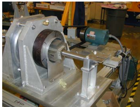
Figure 3-4: Test rig for verification of end region lamination stack loss calculations.
