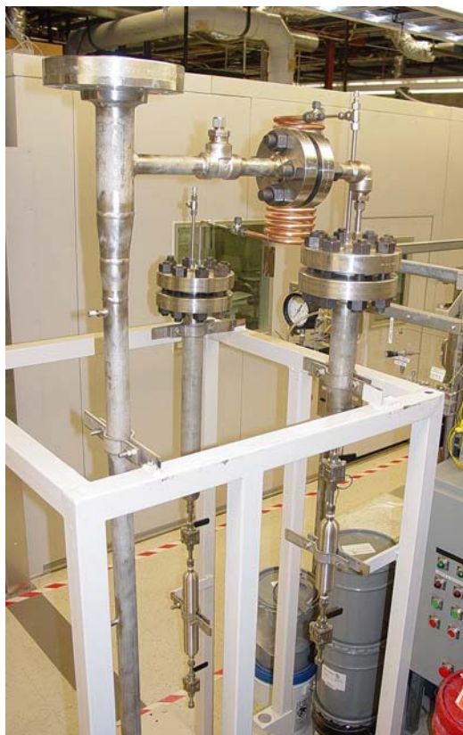
Figure 5. Slurry Bubble Column Reactor and Product Traps
