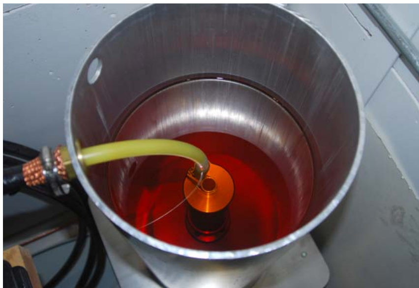
Figure 95. The load tank contains the resistive termination for the discharge chamber. The load is a solid resistor of the type which has been shown to maintain a pure resistance to a fraction of a nanosecond.
