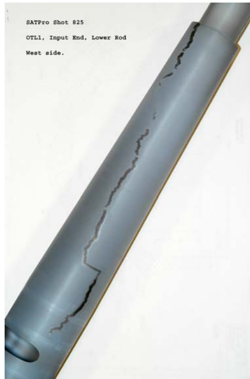
Figure 103. The damage along the rod after a surface failure.
