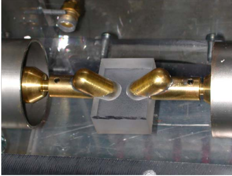
Figure 11. View of electrodes buried in Lexan.
