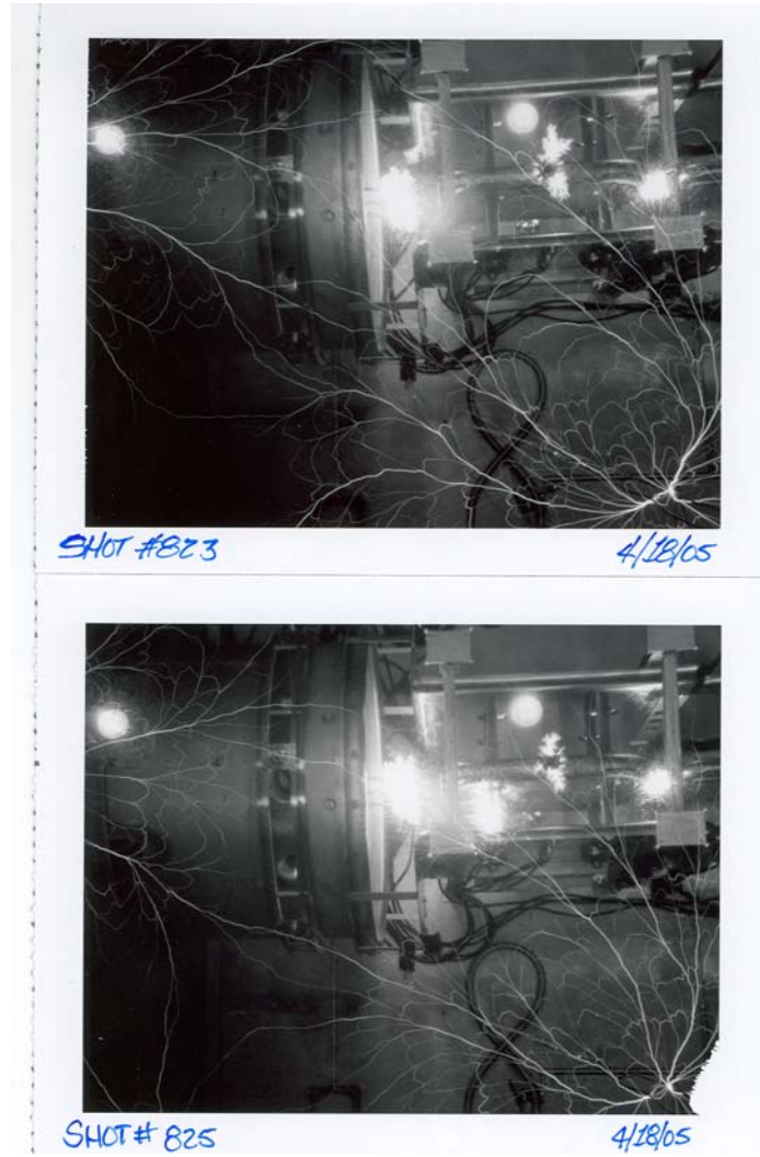
Figure 102. Open shutter pictures showing normal operation (upper) for multimegavolt voltages and a failure along the support rod in the output transmission line section.
