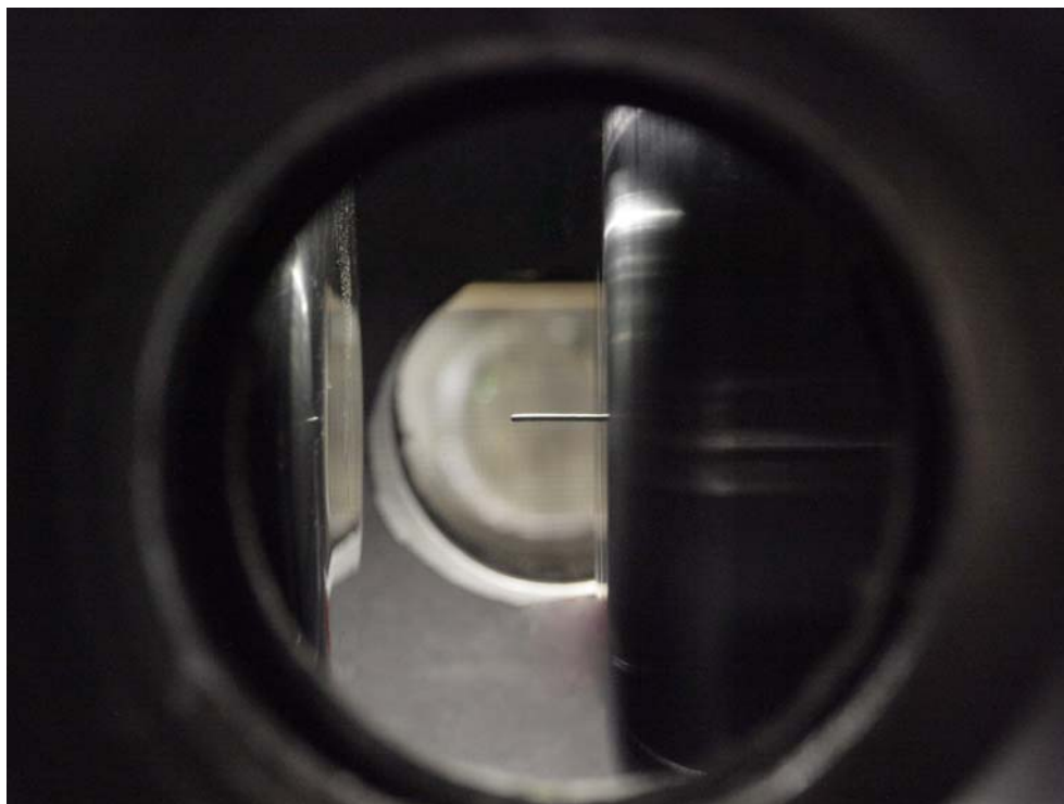
Figure 127. The test gap. The electrodes are identical with the exception of the pin.
