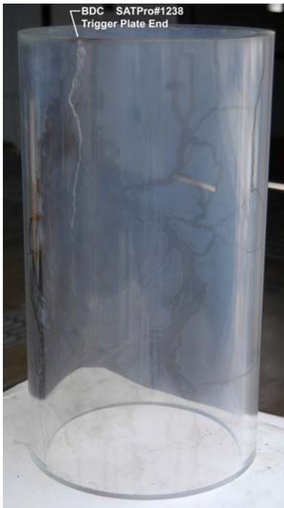
Figure 7. Damage to the dielectric housing caused by surface flashover.
