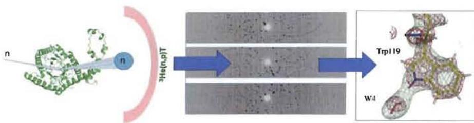
If crystals are of suitable size (> 0.4mm<sup>3</sup>), data can be collected at PCS at LANSCE. As we use time-of-flight Laue techniques, less data is needed for a complete structure, thus overcoming the long (~20h) exposure time. Data is processed and refined with in-house modified software based on D\*trek and CNS.
