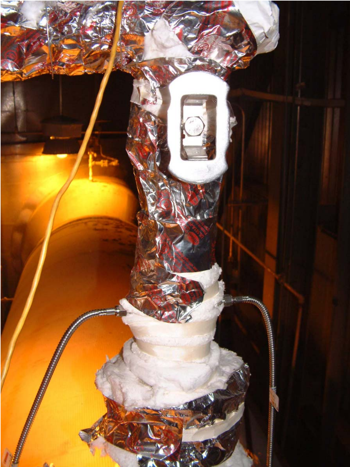
Figure 4. Upper portion of the heated, insulated GTI sample probe showing the handle of the shutoff valve.
