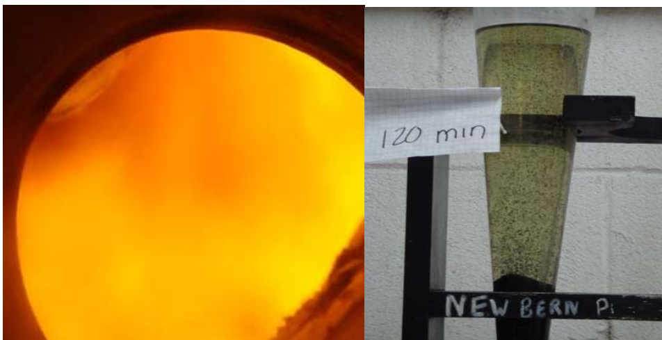
Figure 4-13 The flame picture is taken approx 15.00 2008-mar-06. The flow rate is 50 gpm black liquor and the nozzle pressure in the 25-30 psig range. Typical Imhoff cone after 2h in the New Bern Mill, the picture is from 21-Feb-2008
