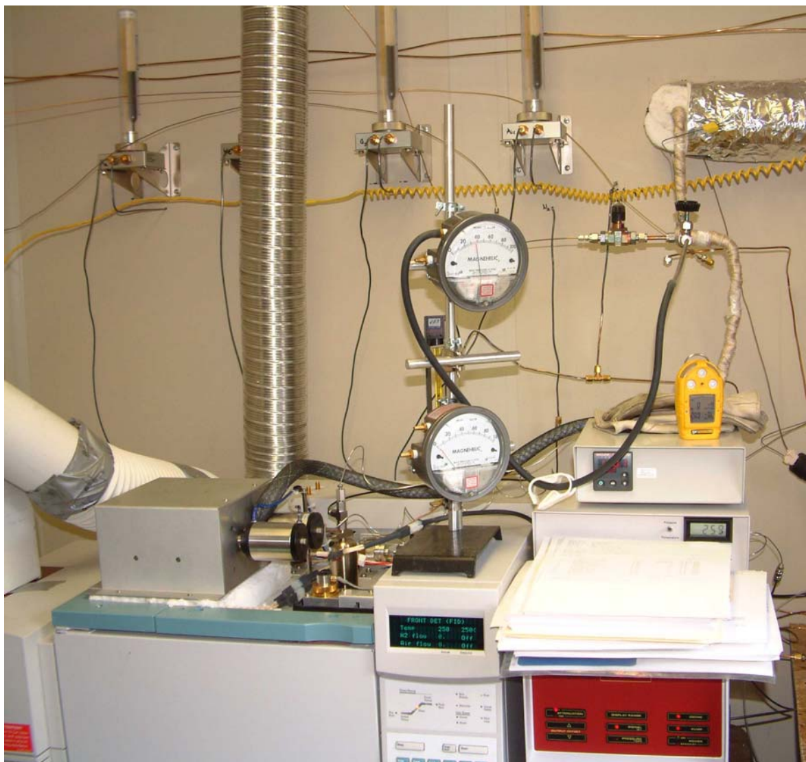
Figure 12. Distribution of calibration gases to the GC/MSD/FID/SCD system.
