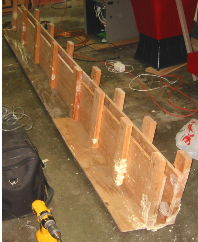
Figure 6-1: Form for Extrusion Foaming Process
