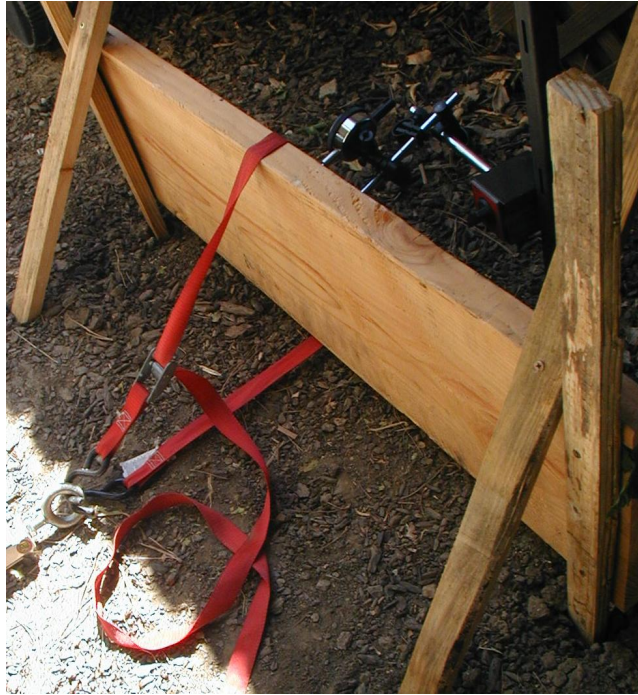
Figure 6-7: Traditional Method Deflection Testing
