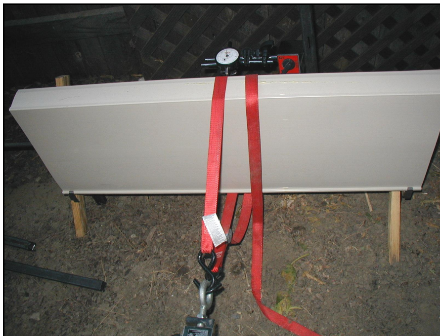
Figure 6-6: E-Form System Deflection Testing
