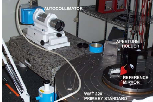
Figure 2: Measurement set-up for the calibration of electronic autocollimators against the PTB angle comparator Heidenhain WMT 220. The autocollimator measures the angle of a plane mirror attached to the comparator's rotor unit. The autocollimator is rotated by 90 degrees to align its main measuring axis for the DLTP application (y-axis) with the comparator's horizontal plane of rotation. The comparator is located in a clean-room laboratory. The lab is kept at a highly stable ambient temperature ( \Delta T < 0.05 K), a constant laminar air flow ( v = 20 cm/s) and very small floor vibrations.
