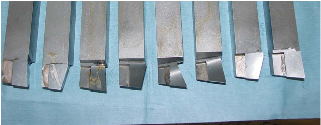
1. Variations in Side Rake, Special Brazed Tip Tools (3, -6, 6, -6, 12, -9, -6, 6)
