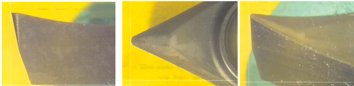
Side Top Cutting Edge 3. Multiple Views of the Kennametal DPGT3251HP Insert (high rake w/integral chip breaker and sharp cutting edges)
