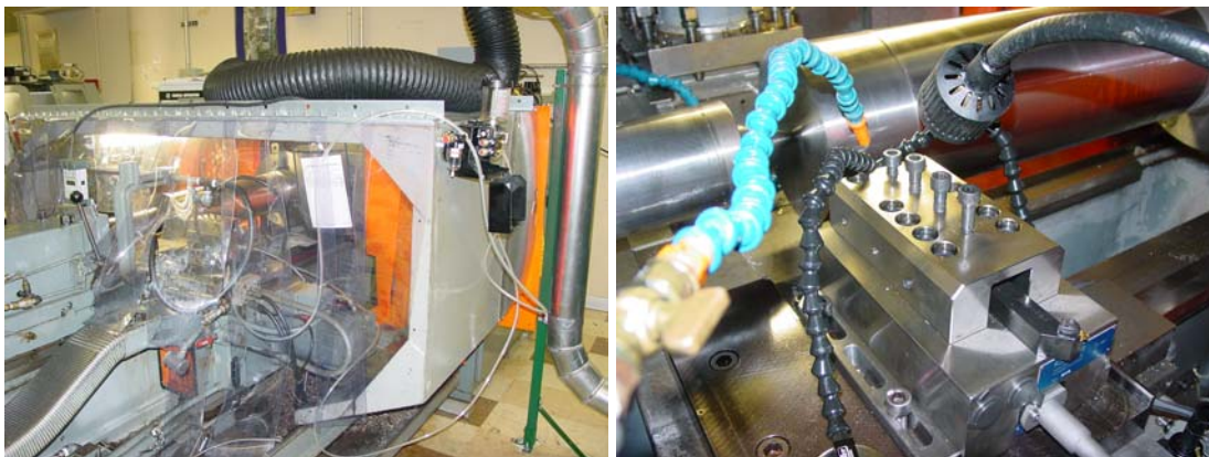
6. Splash Shield Modified to Control Mist
