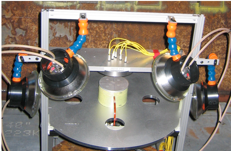
Figure 1. Example (2021E PT3) of shot stand with PDV probes sighted on diagnostic plate
