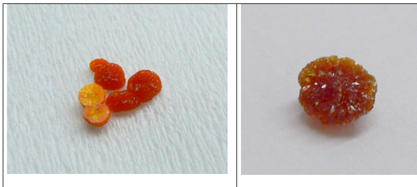
Figure 3.4 Uranium solids containing aceto-hydroxamic acid produced at low nitric acid concentration
