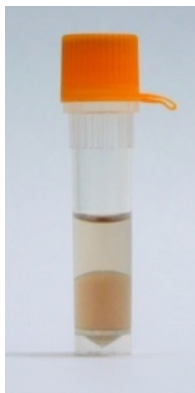
Figure 7.2 Characteristic brownish-red color of Pu(IV)-AHA complex suggest its presence in TBP after extraction of Pu(IV) from HNO 3 in the presence of AHA.
