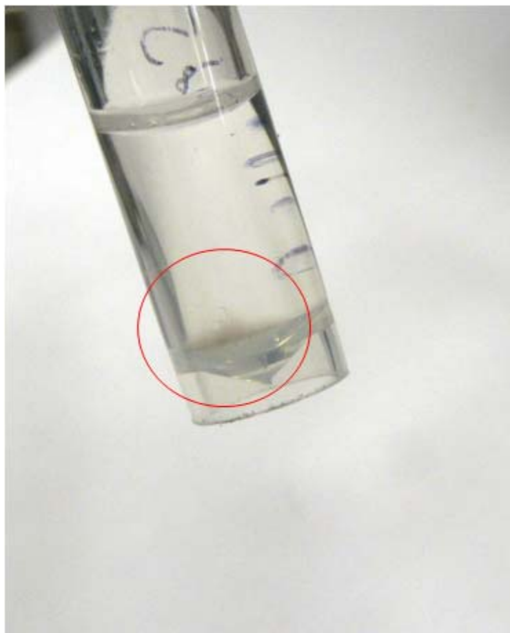
Figure 6.5 Picture of Pu colloid in TBP formed after extraction from 0.1 M \text{HNO}_3 and centrifugation of the organic phase.
