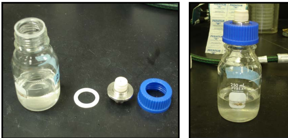
Figure 3. Gas-tight bottle sealed with metal port fittings and capped with a white plastic septum underlain with an additional silicone septum.
