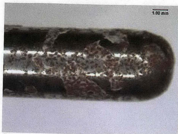
Figure 8. The appearance of the sample after CPP testing in deaerated 270-LT simulant at 50°C
