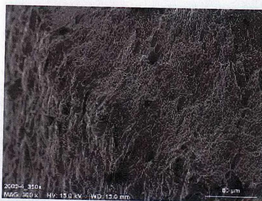
Figure 10. A stereo micrograph of the sample from the test performed in modified AN107 (0.35 M nitrite, 3.5 M nitrate) at 50°C and at OCP (-254 mV vs. SCE).
