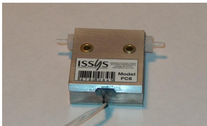
Figure 18: Photo of Fuel Concentration Sensor
