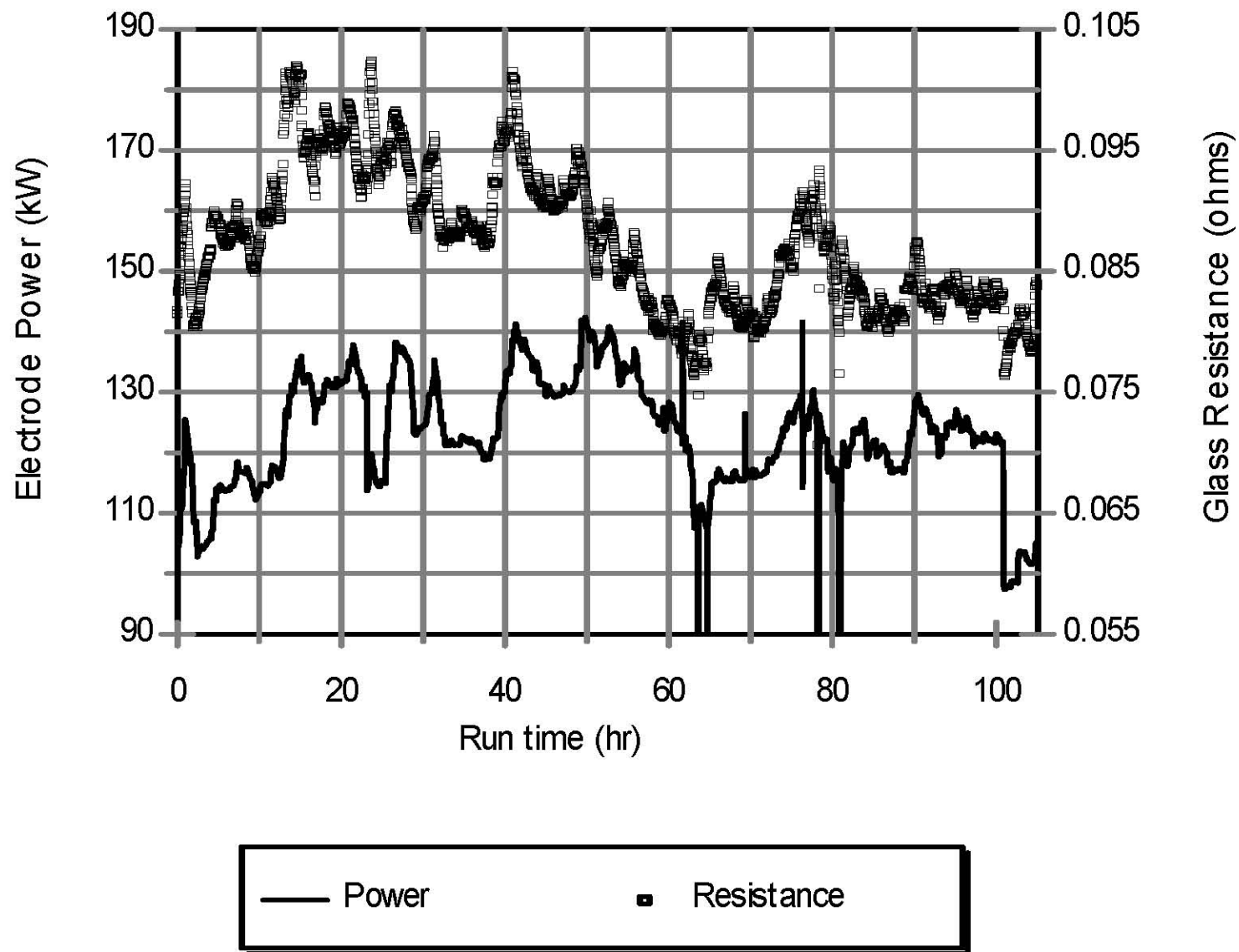
Figure 5.6.b. Electrode power and glass resistance for DM1200 Tests 2 and 3.
