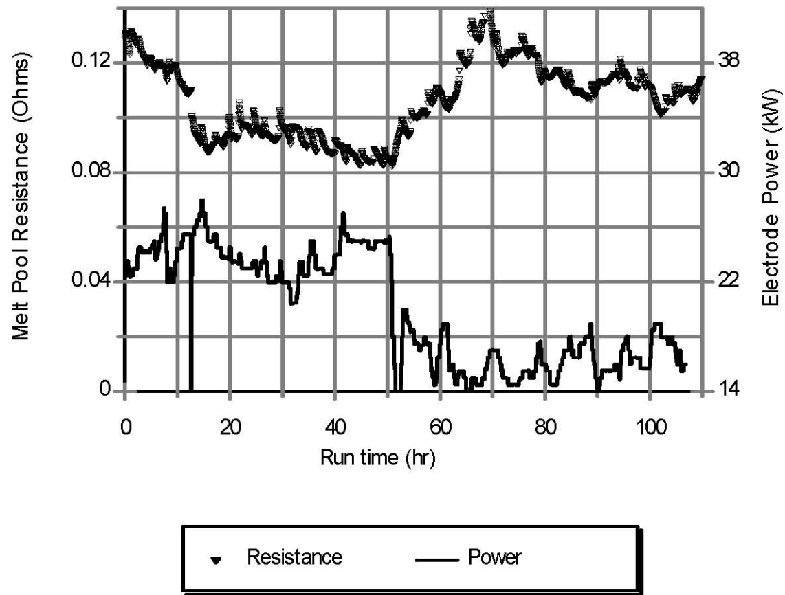
Figure 4.6.c. Melt pool resistance and total electrode power during DM100 Tests 5 and 6.
