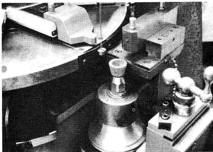
FIGURE 4 - View of semiautomatic grinder showing vertical spindle, grinding wheel and vacuum head.
