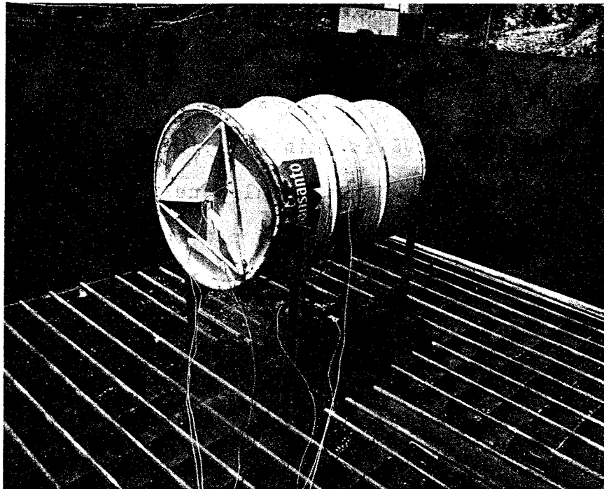
Figure 1 - Thermal Test Setup, early prototype test. This test setup, with the air manifold and 16 sheet metal block-out boxes, was used to abate the smoke in the aviation gasoline fire to the levels demonstrated in figures 2 and 3.
