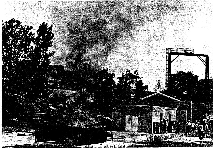
Figure 2 - Thermal Test Area, early prototype test. This view shows the results of early fire tests with 1000 ft 3 /min (STP) of air added to the fire.
