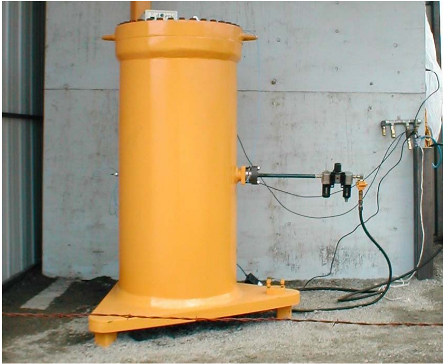
Figure 22. EGS1 test rig with shock tube and receiver
