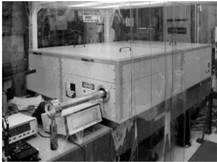
Figure 7 The LLNL Laser Peening System.
